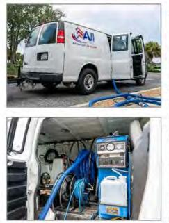
For carpet cleaning at these locations, AJI will be using a van equipped with a CDS 4.8 truck mounted, van-powered cleaning system from HydraMaster. These systems feature OverDrive™ Power Train Technology which allows us to deliver a deep clean to your facilities. The system is equipped with two solution outlets for dual wand capability, three speed settings and a 100 gallon recovery tank for uninterrupted cleaning.
